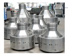
Perfect bowl balancing thanks to sophisticated monitoring and recording systems are used for both high and low speed balancing to reduce at minimum the strength over the mechanical drive. High Quality materials which ensures top strength and very good corrosion resistance.
