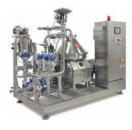
Centrifugation is the most economical polishing and filtration technique. Beer losses are reduced and the organoleptic qualities of the beer are protected. REDA centrifuges are sealed with a liquid ring to avoid any risk of oxidation of the product. The life span of the filters after the centrifuge is considerably extended.
